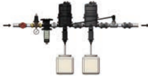
dual remote injection installation
